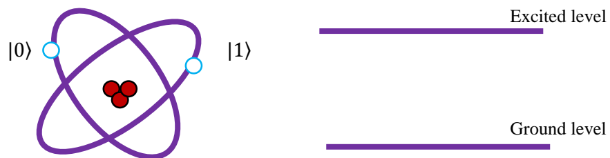
Qubit represented by two electronic levels in an atom
